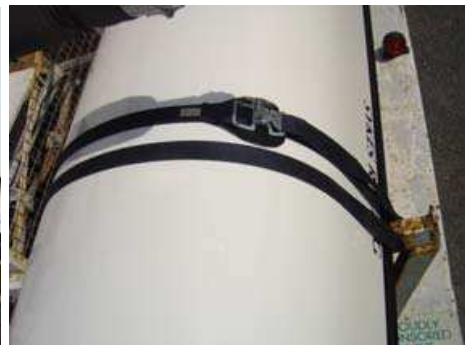
Buckle too high Wrong!
